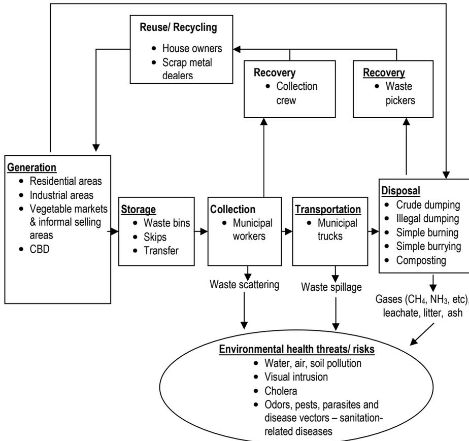
**Figure 1 The Functional Components of Chinhoi's Waste Management System**
